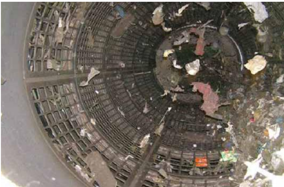
Figure 2: Waste separation using a trommel screen
